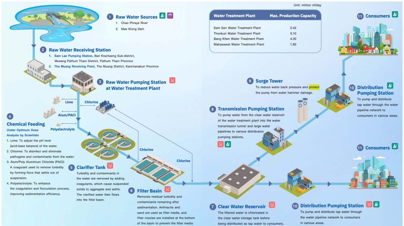
Figure 2: The Water Production Process
