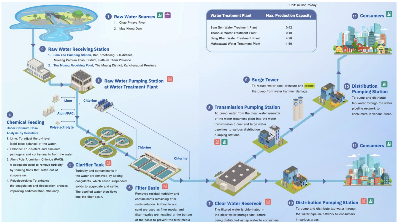
Figure 2: The Water Production Process
