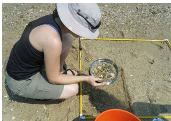
Figure 4.13 Sampling surficial beach sediments for meso-plastics, using a one metre square quadrat and a hand-held stainless steel sieve, Calvert Cliffs and Cove Point (© NOAA Marine Debris Program).
